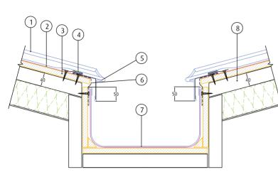
2 Slope box gutter
