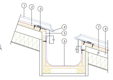
Slope box gutter
